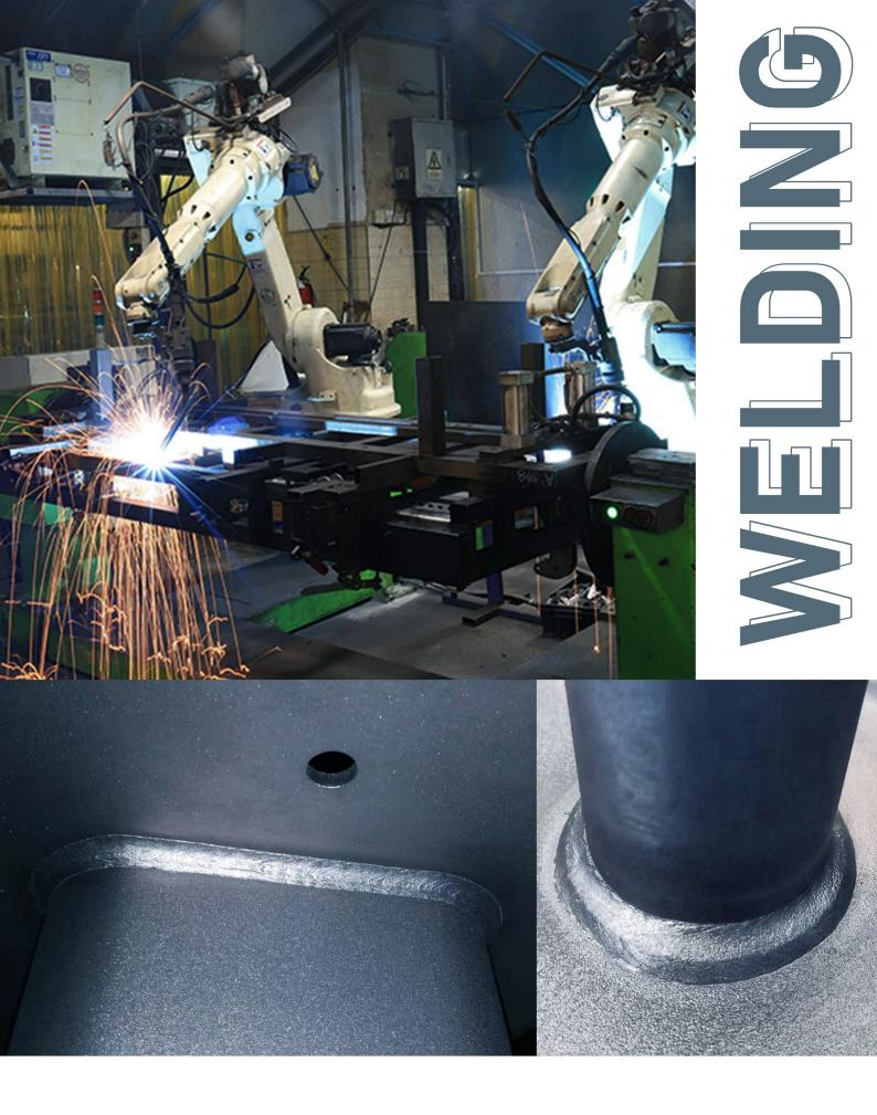
Automatically welding technologies including double-slide table welding group, cluster welding group, double-station welding group
